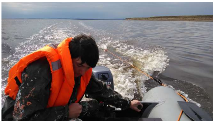
Figure 2. Continuous resistivity profiling at the river.
