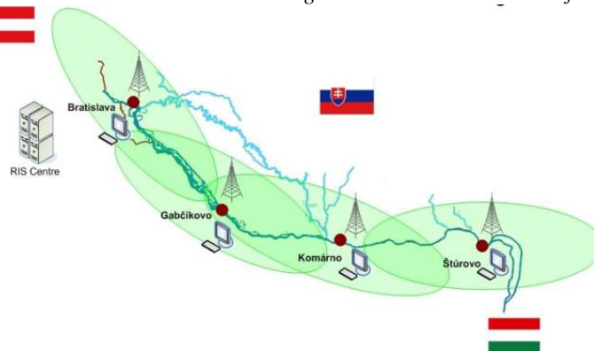
Figure 1: Base shore stations and the AIS signal on the Slovak stretch of Danube
