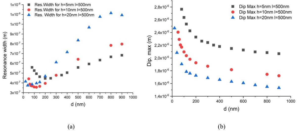
**FIGURE 4.** (a) the dependence of the width of the resonance on the width of the nanobaulk  $d$  at  $h = 5, 10, 20$  nm; (b) the dependence of the value of the resonance wavelength on the width of the nanobaulk  $d$ .
