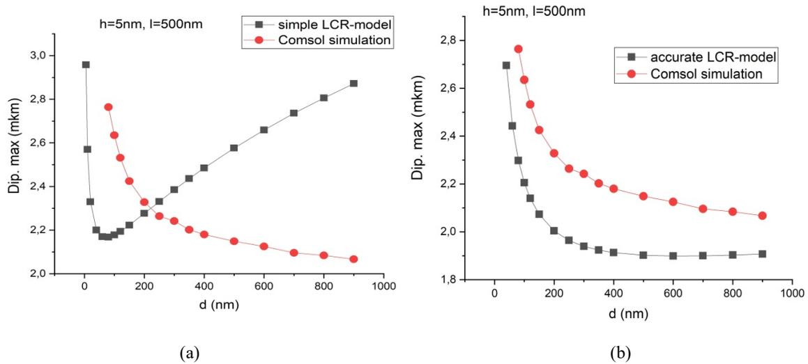
**FIGURE 5.** Dependence of the value of the resonant wavelength on the width of the nanobauk  $d$  for full-wave calculation and the simplified formula of the LCR model
