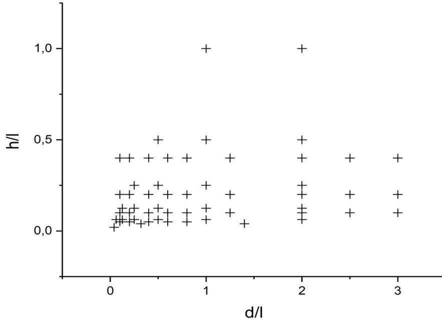
**FIGURE 2.** The range of nanobaulk shape factors in which the approximation (11) and (12) is checked by simple analytical formulas of integrals for inductance L and capacity C.
