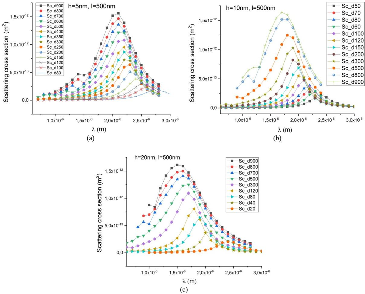
**FIGURE 3.** Scattering cross section depending on the incident radiation wavelength: (a) for  $h=5\text{nm}$ ; (b) for  $h=10\text{nm}$ ; (c) for  $h=20\text{nm}$ .
