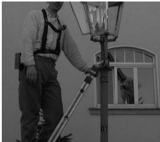
FIG. 1. Personal air monitoring during maintenance of gas lanterns.
