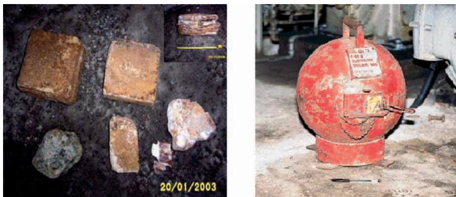
FIG. 2. Pieces containing radioactive material identified in a Spanish metal recycling facility by applying the working procedure of the protocol.
