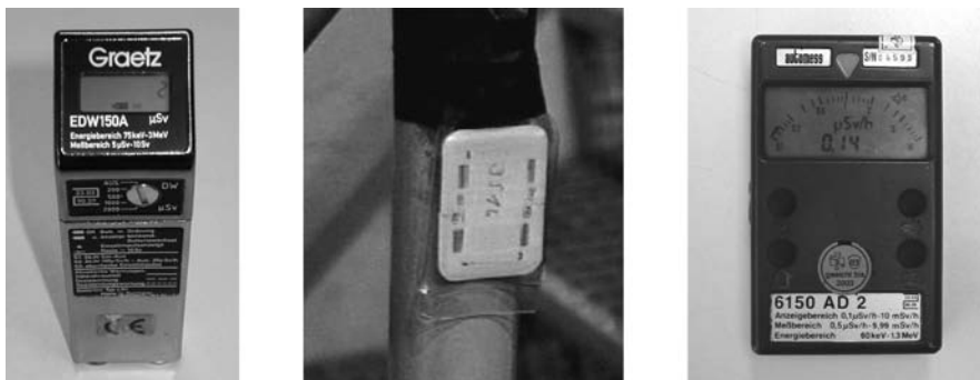
FIG. 2. Measuring equipment: EPD, TLD (installed at shear exit) and area dose rate meter.
