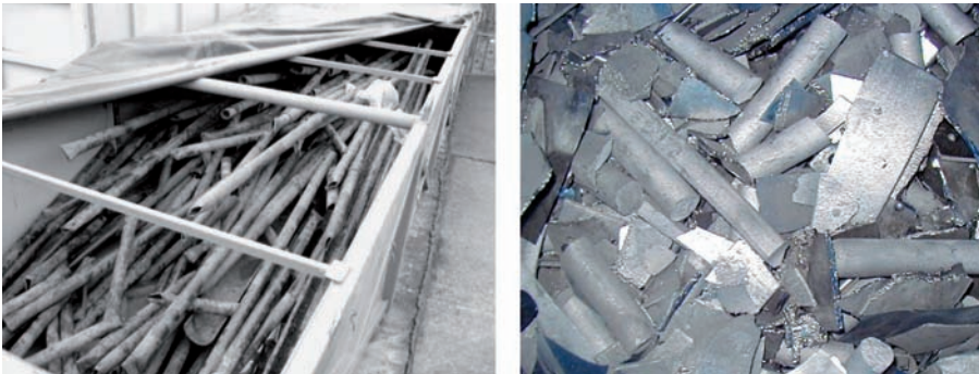
FIG. 1. Examples of contaminated pressure pipes from the oil and gas industry and waste material from the tungsten welding electrode industry.
