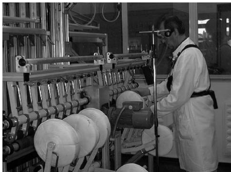
FIG. 2. Personal air monitoring during the drying of coils.
