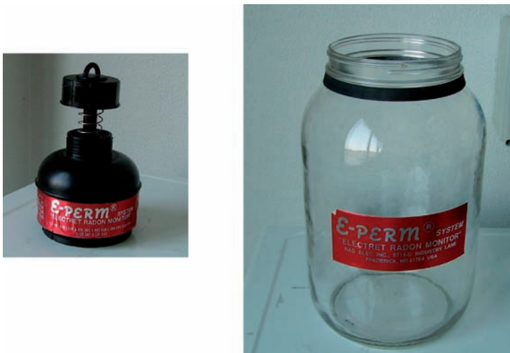
FIG. 3. Electret ion chamber and glass jar of the E-PERM ® system.
