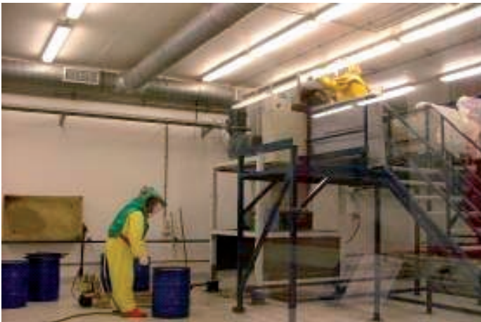
FIG. 6. Shredding of filters in the AVG.
