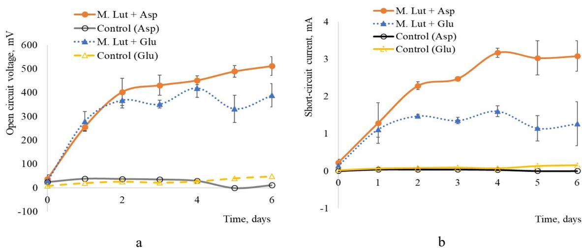
**Figure 2.** Dynamics of open circuit voltage (a), short-circuit current (b) generated in BFC by *M. luteus* 1-I strain when using aspartic (0.5 g / l) and glutamic (0.5 g / l) acids.
