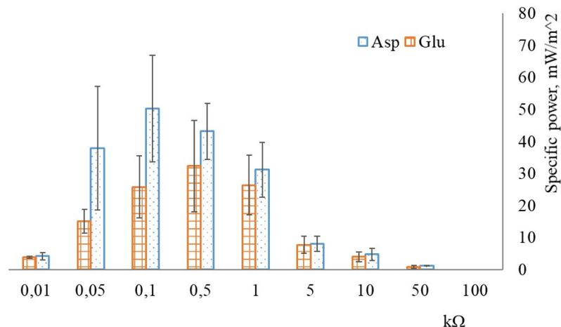
**Figure 3.** Specific power indicators of BFC based on *M. luteus* 1-I strain using aspartic (0.5 g / l) and glutamic (0.5 g / l) acids, measured at resistance in the range from 0.01 to 100 k $\Omega$ .
