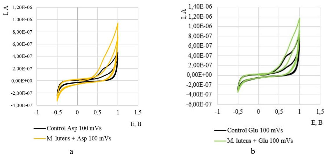
**Figure 6.** Cyclic voltammograms measured in solutions of dicarboxylic amino acids in the presence of *M. luteus* 1-I strain (potential sweep rate 100 mV/s)
