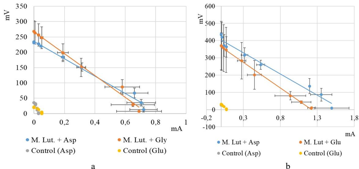
**Figure 4.** Current-voltage characteristics of BFC based on *M. luteus* 1-I strain when using aspartic (0.5 g / l) and glutamic (0.5 g / l) acids on the first (a) and fourth (b) days of the experiment.
