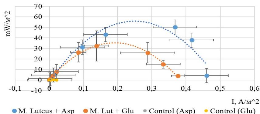
**Figure 5.** The ratio of the specific power (mW / m<sup>2</sup>) to the specific strength (A / m<sup>2</sup>) of the BFC current based on the *M. luteus* 1-I strain when using aspartic (0.5 g / l) and glutamic (0.5 g / l) acids on 4 days of exposure (4th day).
